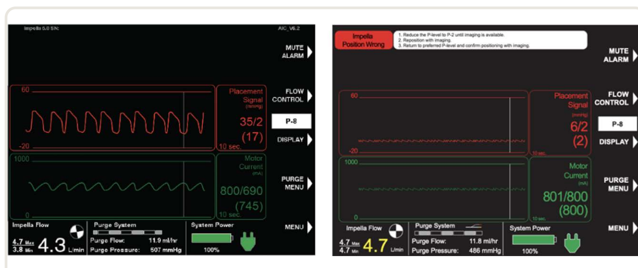
Fig. A1. Placement screen. Placement screens generated by a differential pressure sensor (Impella LD and 5.0) in an appropriately placed transvalvular heart pump ( left ) and inappropriately placed transvalvular heart pump ( right ) are shown. ( Right ) The inlet and outlet areas of the pump are in the same chamber (either the aorta or ventricle), resulting in no pulsatility in the placement signal or motor current. Adapted and reproduced with permission from Abiomed Inc. (USA).
